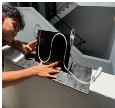
Fig. 3. The operator unlocks the zero-play brass hinge, carefully drops the board to 60°, logs the data
