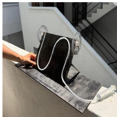
Fig. 4. The operator unlocks the zero-play brass hinge, carefully drops the board to 45°, logs the data
