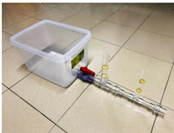
Fig. 2. Complete venturi meter experimental setup
