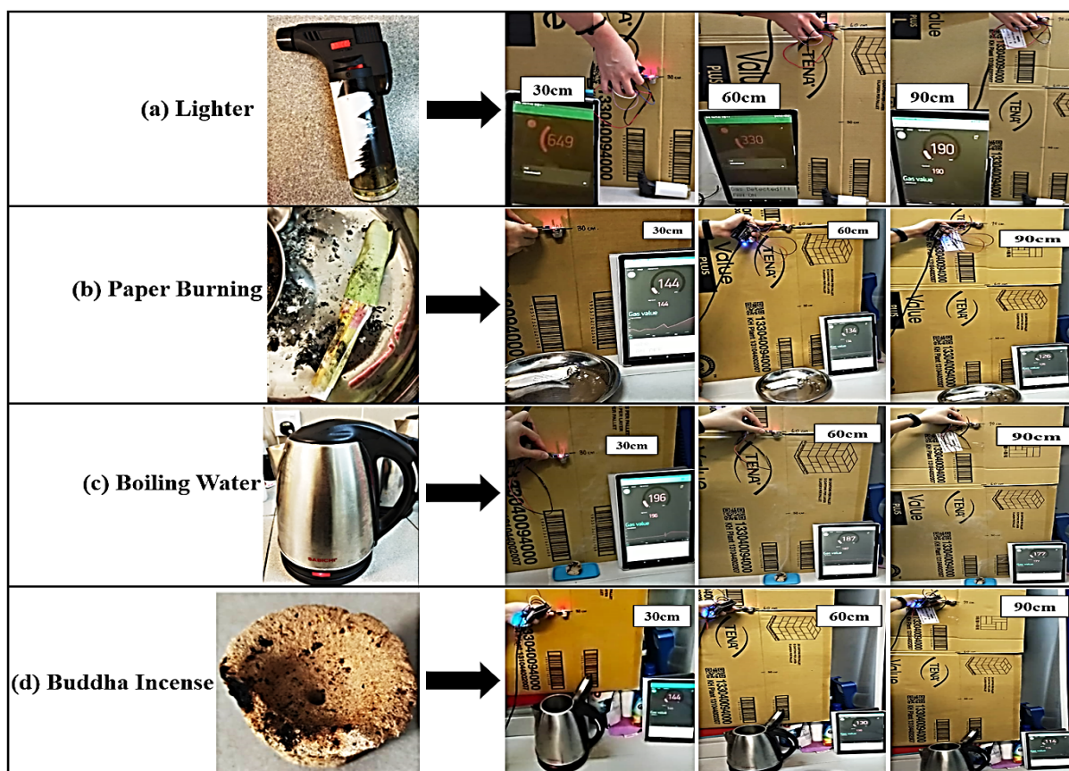
Fig. 15. Gas detection at different sensor placement distances
