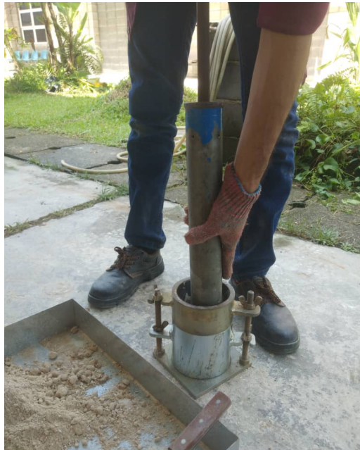
Fig. 4. Standard Proctor test
