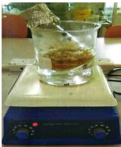
Fig. 2. Hot water extraction using double boiling method
