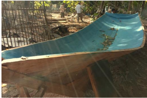
Fig. 5. Part of constructed boat body without frame
