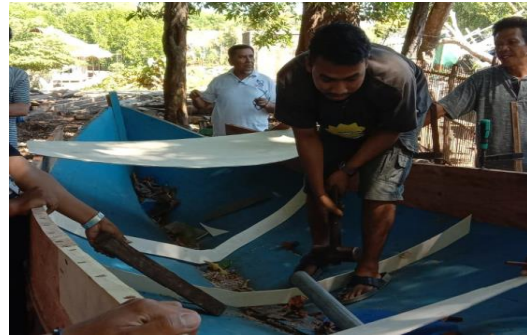
Fig. 6. Frame pattern making
