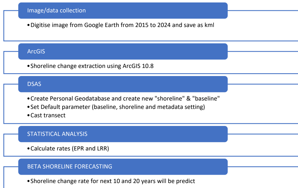
Fig. 3. Flow chart of data collection and processing using DSAS
