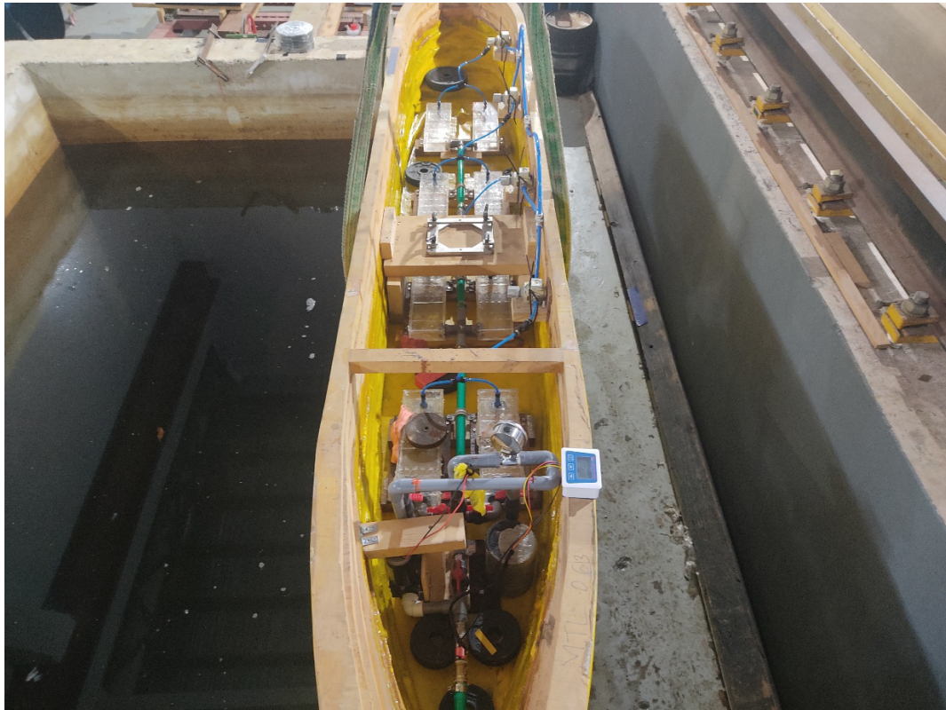
Fig. 5. Perspective view of MTL 063 equipped with BFS system
