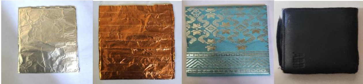
Fig. 5. RFID Cards wrapped in (a) Aluminium Foil (b) Copper Roll Sticker (c) Envelope Paper (d) Synthetic leather
