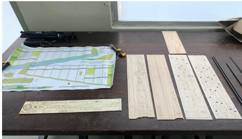
Fig. 2. Shaka glider components
