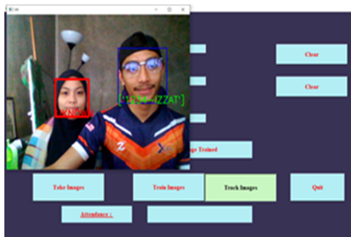
Fig. 8. Screen displaying registered passengers indicated in green, whereas unknown persons in red
