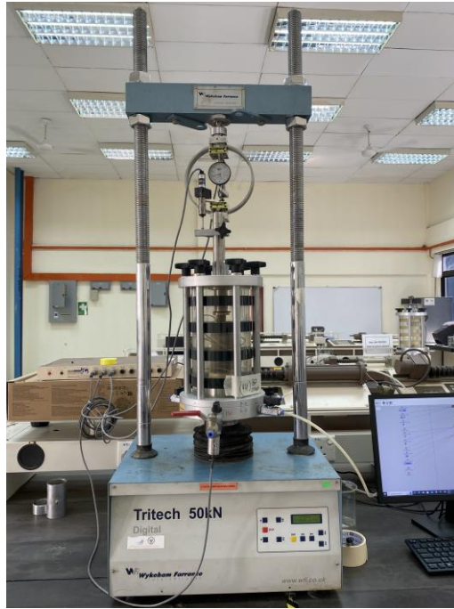
Fig. 1. Triaxial Test – Unconsolidated Undrained set up
