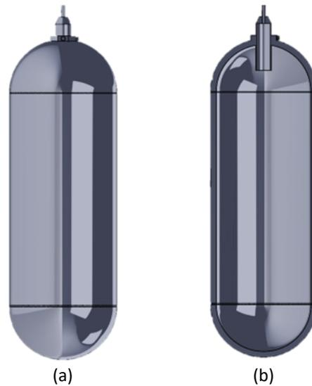
**Fig. 2.** Tank design (a) Front view (b) Cross-sectional view
