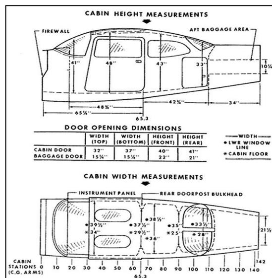
**Fig. 1.** Cabin height and width measurements of the Cessna 172 [20]
