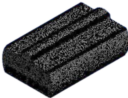
Fig. 3. Mesh generation of the aircraft cabin model
