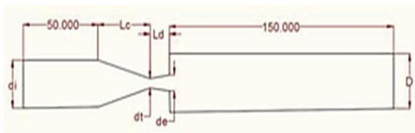
Fig. 3. Geometry of nozzle and enlarged duct by Khizar Ahmed Pathan
