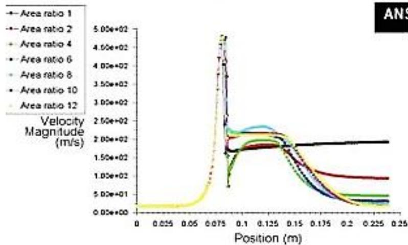
**Fig. 1.** Velocity distribution along the axial length for NPR = 2.0 at different area ratios
