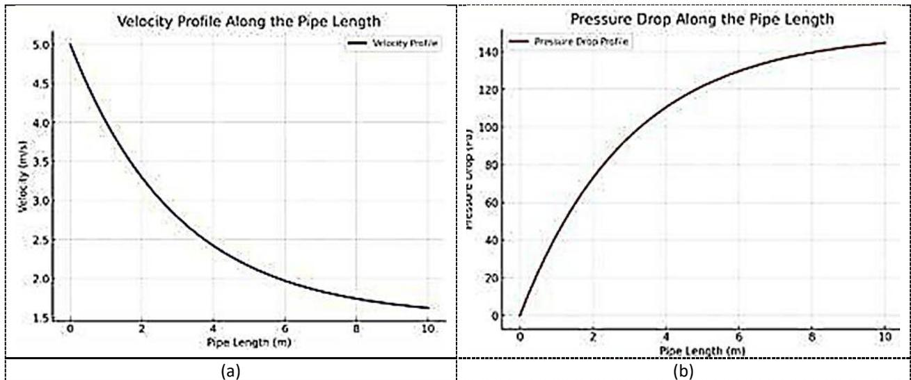
Fig. 2. Comparison along the pipe length (a) Velocity (b) Pressure drop
