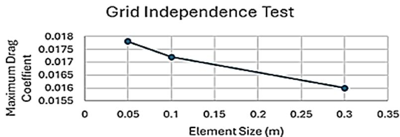
**Fig. 3.** Grid independence test
