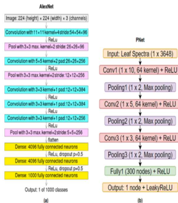
Fig. 2. (a) AlexNet architecture (b) PNet architecture
