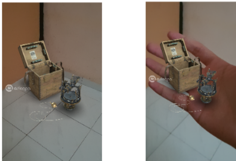
Fig. 2. Object rendering and occlusion test on device without LiDAR
