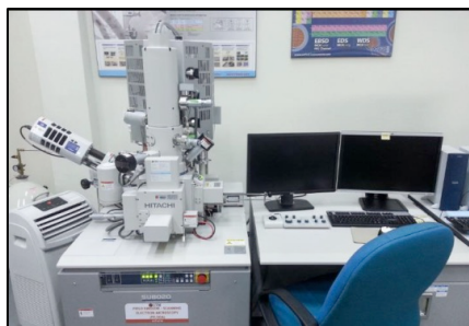
Fig. 3. Hitachi Scanning Electron Microscopy (SEM) with Energy Dispersive X-Ray (EDX)
