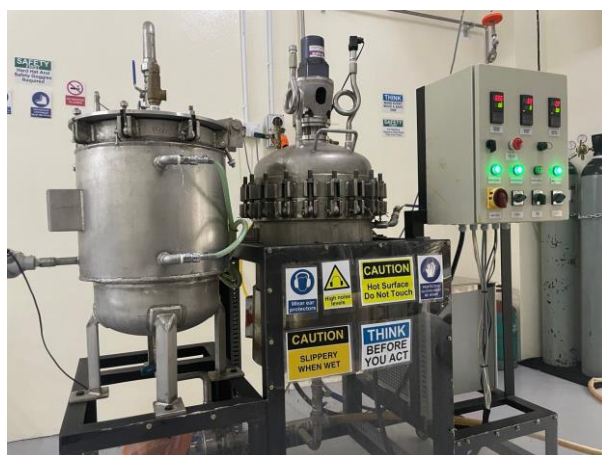
Fig. 1. Industrial scale subcritical water extractor by AM Zaideen ventures Sdn. Bhd.
