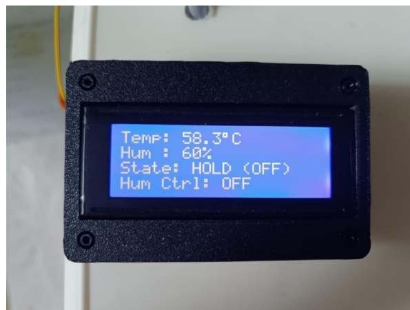
Fig. 11. LCD showing humidity control in the "Off" state
