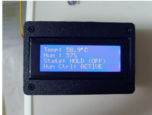
Fig. 7. Humidity control in the "Active" state (below 75% RH)
