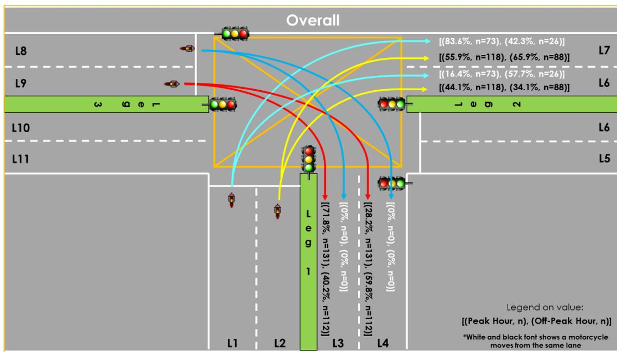
**Fig.5.** Motorcycle Path for Turning Movement
