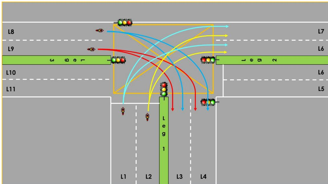
**Fig.4.** Observing Motorcycle Path for Turning Path at Three-legged Signalised Junction
