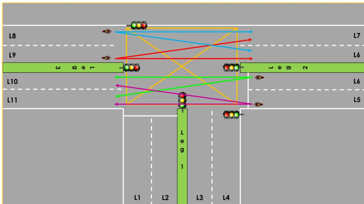
**Fig.3.** Observing Motorcycle Path for Straight Path at Three-legged Signalized Junction
