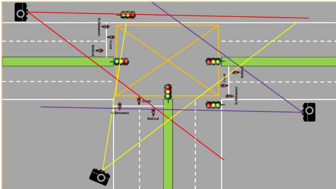
**Fig.2.** Visual of Video Camera Positioning During Data Collection
