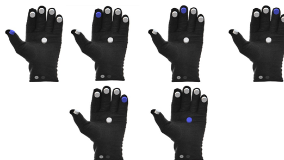
Fig 3. Haptic globe and traveling sensation sequence
