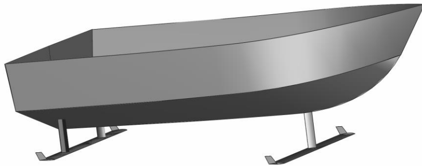
Fig. 1. Hydrofoil craft equipped with winglet
