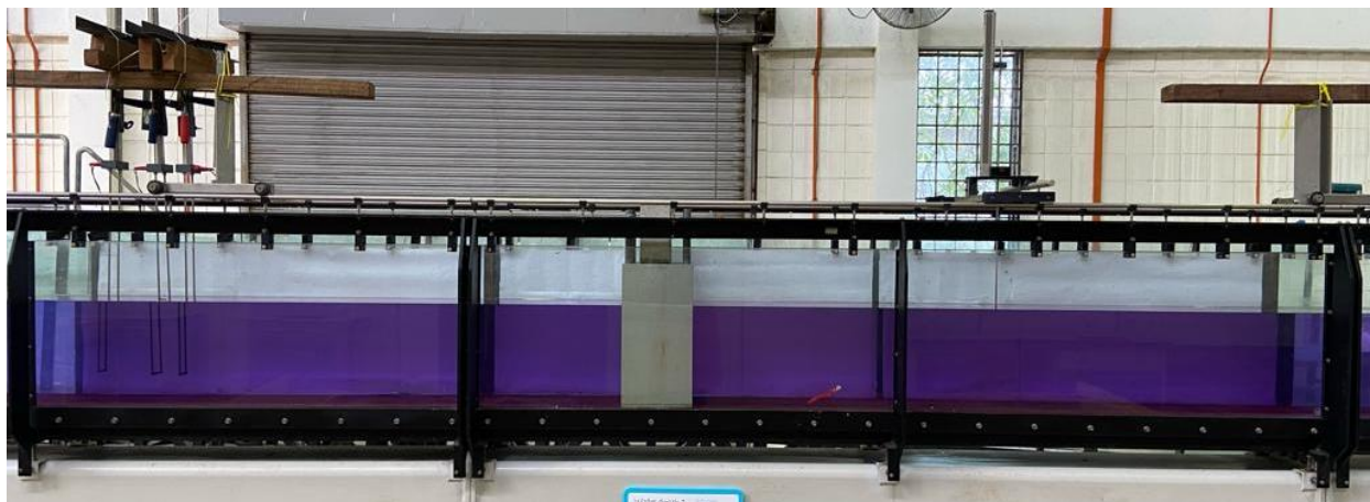
Fig. 9. Breakwater structure in a wave flume with attached wave probes stationed at the back and front of the model
