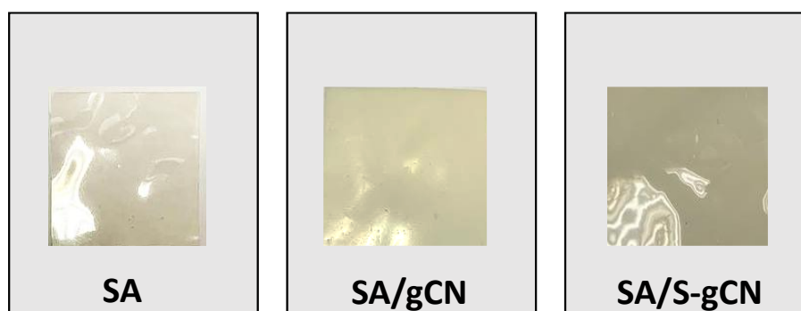
Fig. 3. Physical observation of SA membrane with gCN and S-gCN fillers
