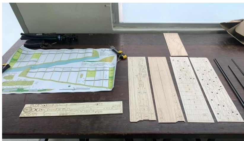
Fig. 2. Shaka glider components
