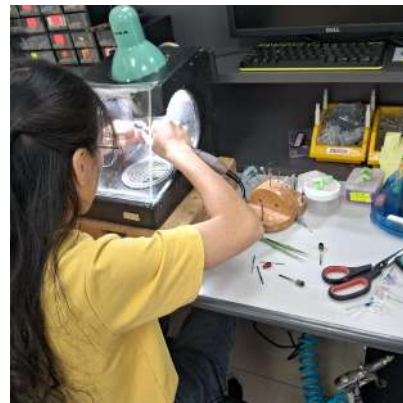
Fig. 7. Earmould modification and trimming
