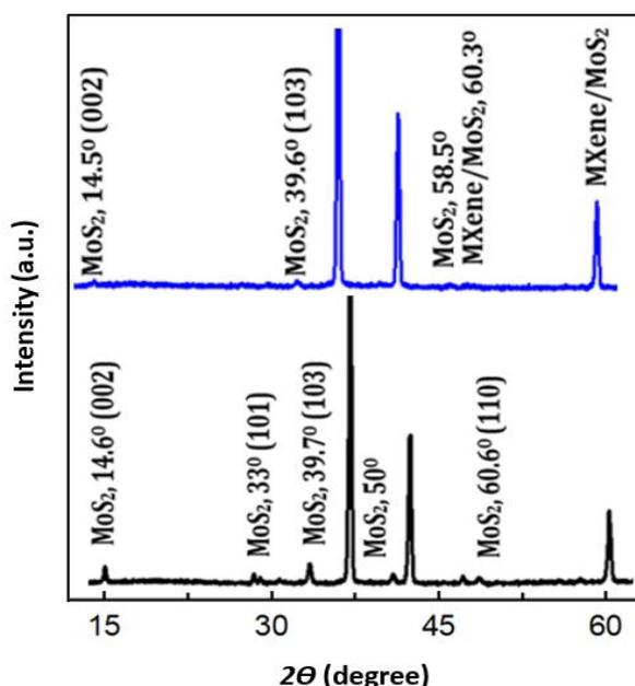
Fig. 5. XRD of MoS<sub>2</sub> and MXene/MoS<sub>2</sub> electrode
