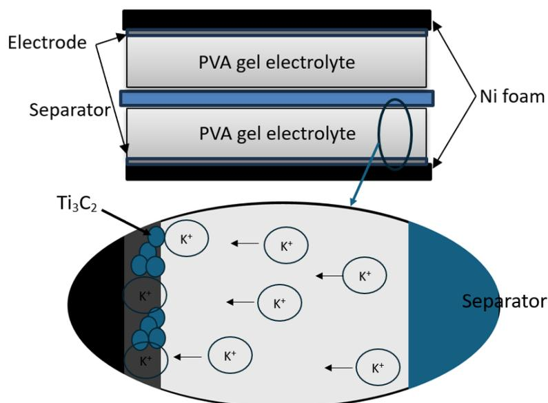
**Fig. 11.** Suggestion for schematic movement of  $K^+$  ion within the electrolyte and their interaction with the current collector
