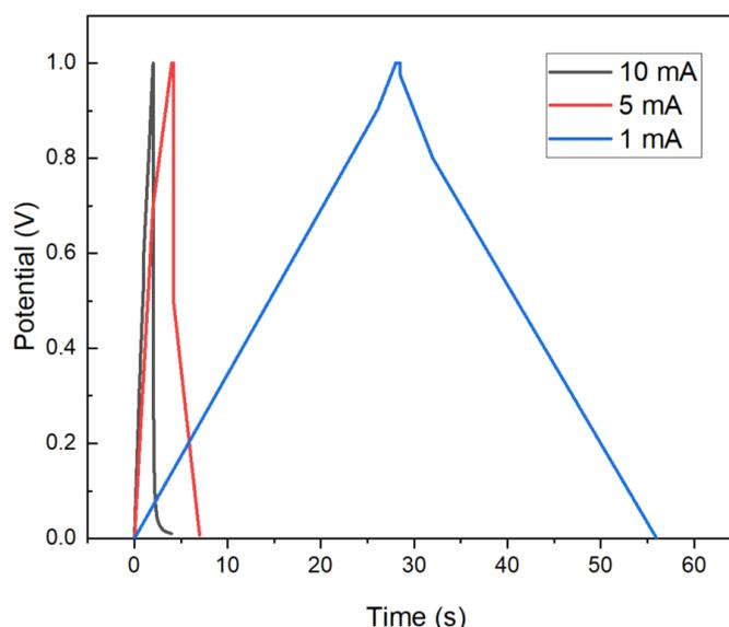
**Fig. 9.** GCD pattern of the MXene/MoS<sub>2</sub> hybrid electrode
