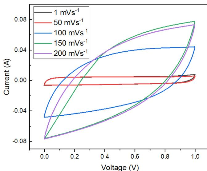
**Fig. 8.** CV curves of the MXene/MoS<sub>2</sub> symmetrical supercapacitor at different scan rates
