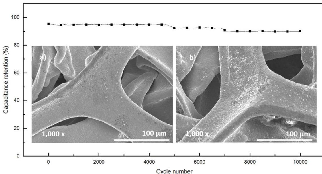
**Fig. 10.** Sample (a) before and (b) after 10,000 cycles capacitance retention evaluation
