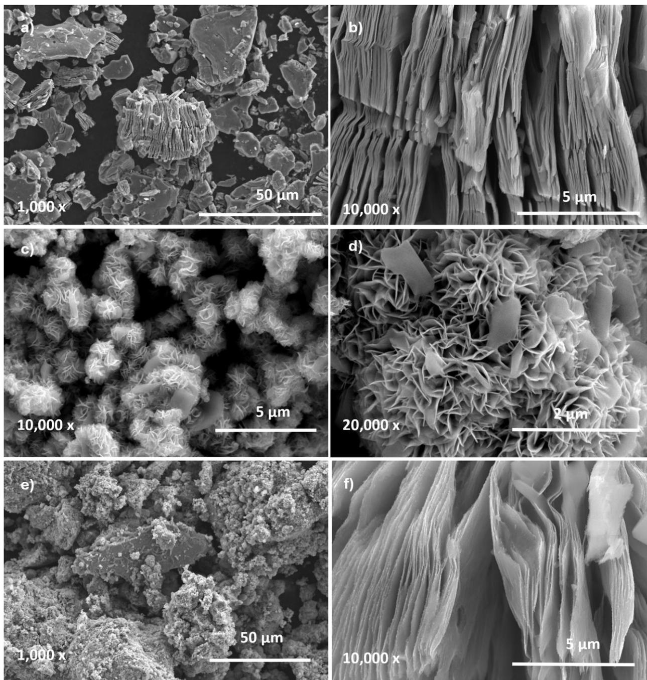
Fig. 6. FESEM images of a), b) Ti<sub>3</sub>C<sub>2</sub> MXene, c), d) MoS<sub>2</sub>, and e), f) MXene/MoS<sub>2</sub> electrode
