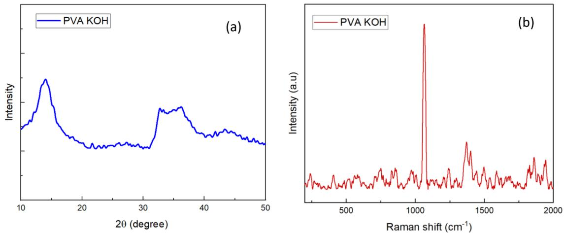
**Fig. 7.** (a) XRD and (b) Raman spectrum of PVA solid electrolyte
