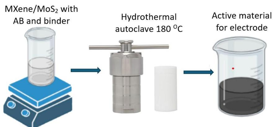
Fig. 4. Schematic representation of hydrothermal synthesis of MXene/MoS<sub>2</sub>
