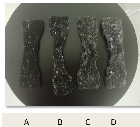
Fig. 8. Failed tensile specimens of TW/RP composites after tensile testing
