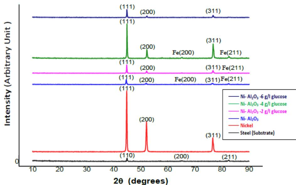
**Fig. 3.** The XRD patterns of steel, Nickel, Ni- Al<sub>2</sub>O<sub>3</sub>, Ni- Al<sub>2</sub>O<sub>3</sub> -2 g/l glucose, Ni- Al<sub>2</sub>O<sub>3</sub> -4 g/l glucose, and Ni- Al<sub>2</sub>O<sub>3</sub> -6 g/l glucose
