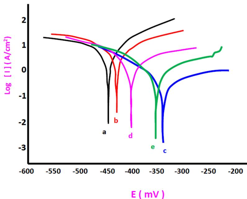
**Fig. 4.** Potentiodynamic polarization curves obtained for (a) Nickel (b) Ni/Al<sub>2</sub>O<sub>3</sub>, (c) Ni/Al<sub>2</sub>O<sub>3</sub> + 2 g/l glucose, (d) Ni/Al<sub>2</sub>O<sub>3</sub> + 4 g/l glucose, and (e) Ni/Al<sub>2</sub>O<sub>3</sub> + 6 g/l glucose, in 3.5% NaCl solution
