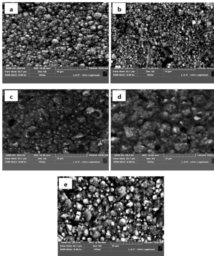
**Fig. 2.** SEM micrographs of the surface morphology of nickel coatings deposited from: (a) Pure Ni (b) Ni- $\text{Al}_2\text{O}_3$  15g/l, (c) Ni-  $\text{Al}_2\text{O}_3$  -2 g/l glucose, (d)Ni-  $\text{Al}_2\text{O}_3$  -4 g/l glucose (e) Ni-  $\text{Al}_2\text{O}_3$  -6 g/l glucose
