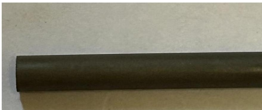
**Fig. 1.** Typical sample after electro-deposition of nickel on steel wire
