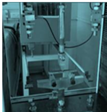
Fig. 5. Flexural Testing Set Up
