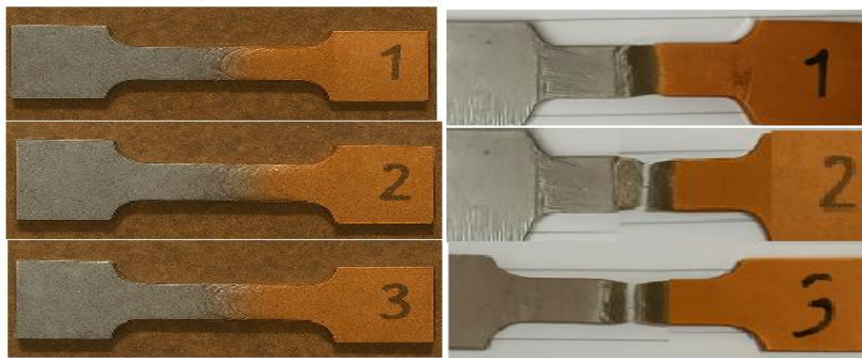
Fig. 4 (a). Specimens for Tensile Testing (b). Specimens after Tensile Testing
