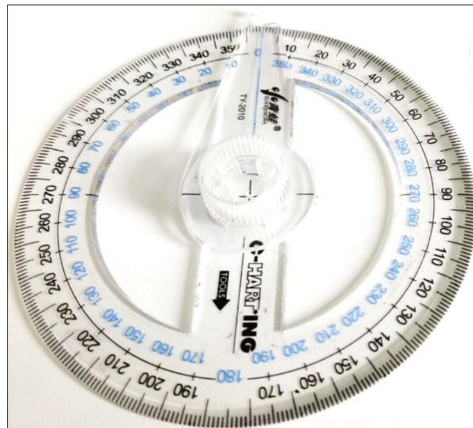
Fig. 6. A protractor used to measure angular bearing
