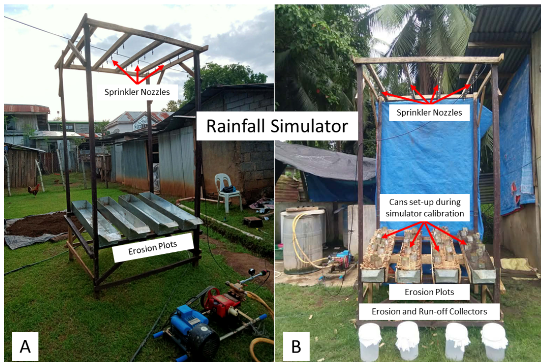
Fig. 1. Constructed rainfall simulator, (A) Attached with erosion plots and (B) Shows the erosion and run-off collectors, cans set-up for during the rainfall simulator calibration.
