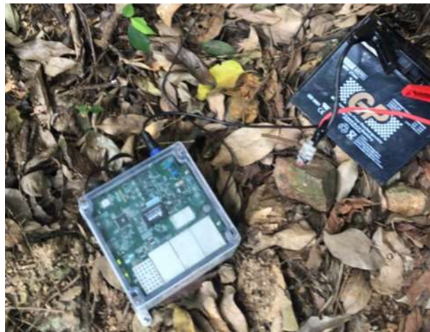
Fig. 1. Seismometer connected to power supply
