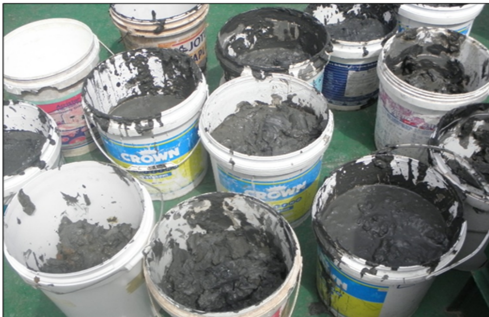
Fig. 1. DMS sample retrieved during dredging activity at Kuala Muda, Kedah, Malaysia
